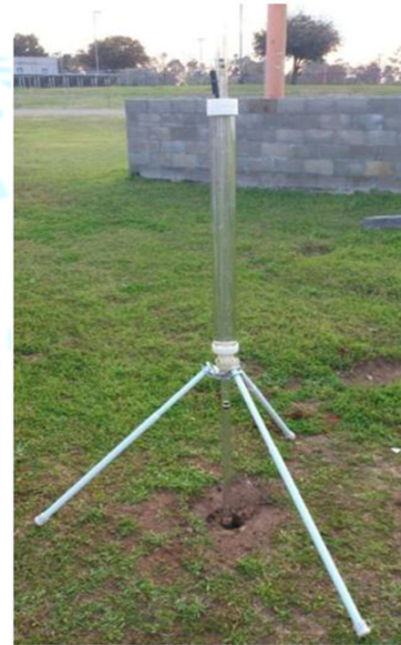
Fig. 2 Guelph permeameter test set-up (Fatehnia, 2015).
